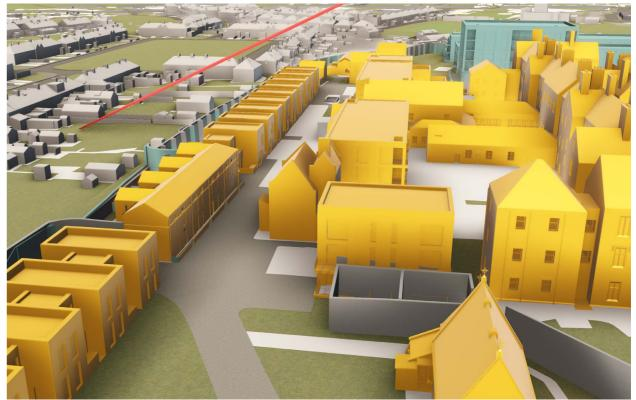
Figure 09: Example of 25-degree angle test
